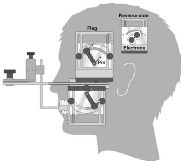
**Fig. 4.** Modified face-bow used for precise relocation of the surface electrodes. Pins and adjustable flags enabled reproducible guidance of the electrodes on to the skin.
