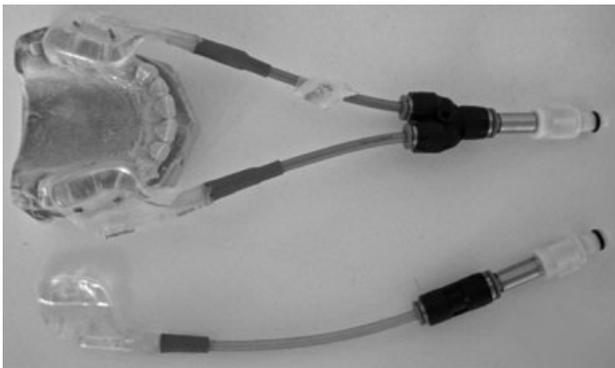
**Fig. 2.** Intraoral device of the measurement system: pressure-sensitive pads mounted on a plastic splint for bilateral biting experiments.
