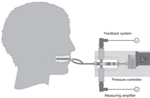
**Fig. 1.** Schematic representation of the hydrostatic pressure-measuring device mounted on intraoral plastic splints.
